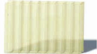
Sample 3 - Delta YI=10 Typical Multiwall Polycarbonate Sheet
