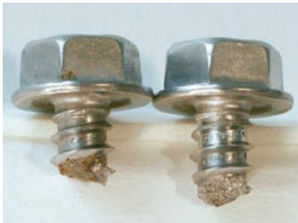
410 SS super passivated fastener with plain finish
