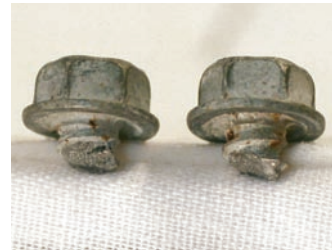
410 fastener with aluminum-filled topcoat
